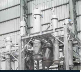
Using a Rising Film Evaporator for pre-concentration and a Thin Film Evaporator as stripper to reduce solvent loss and improve product quality
